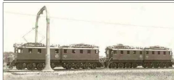
ELECTRIC-POWERED locomotives, with substation-like equipment on their roofs, are shown in service under a cantenary arch on Ford's Detroit, Toledo and Ironton line on July 29, 1928.
