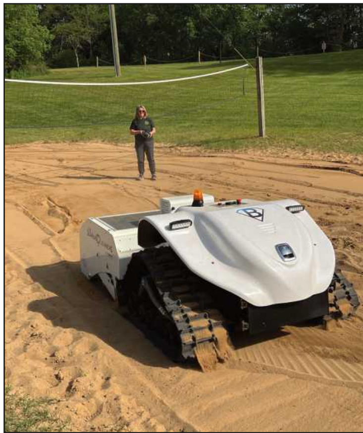
A BE-BOT beach-cleaning robot is operated remotely by Christina Burke, a seasonal worker at Brighton Recreation Area in Livingston County.
