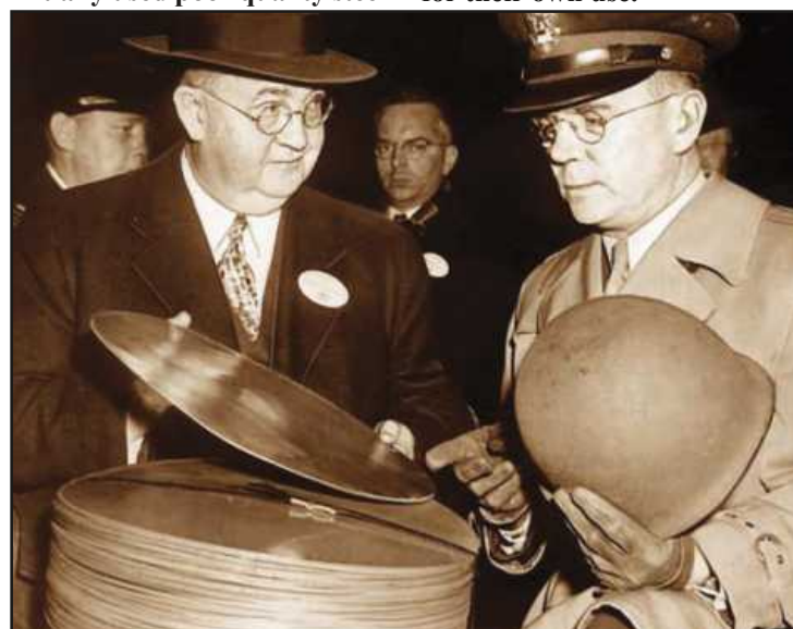
A FLAT DISK OF STEEL that would be stamped into a finished helmet is shown during a military plant tour in March 1943.
