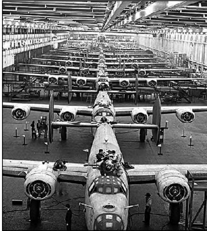
B-24s, SHOWN in production at Willow Run, cruised at 290 mph and carried a 5,000-pound bomb load for 1,700 miles, giving it a longer range, greater speed, and a bigger payload than its B-17 cousin.
